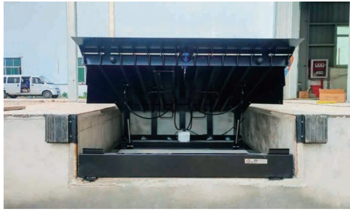
Standard loading and dock leveler
