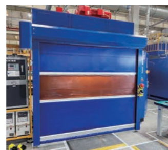
Robotics welding booth anti-arc light protection door
